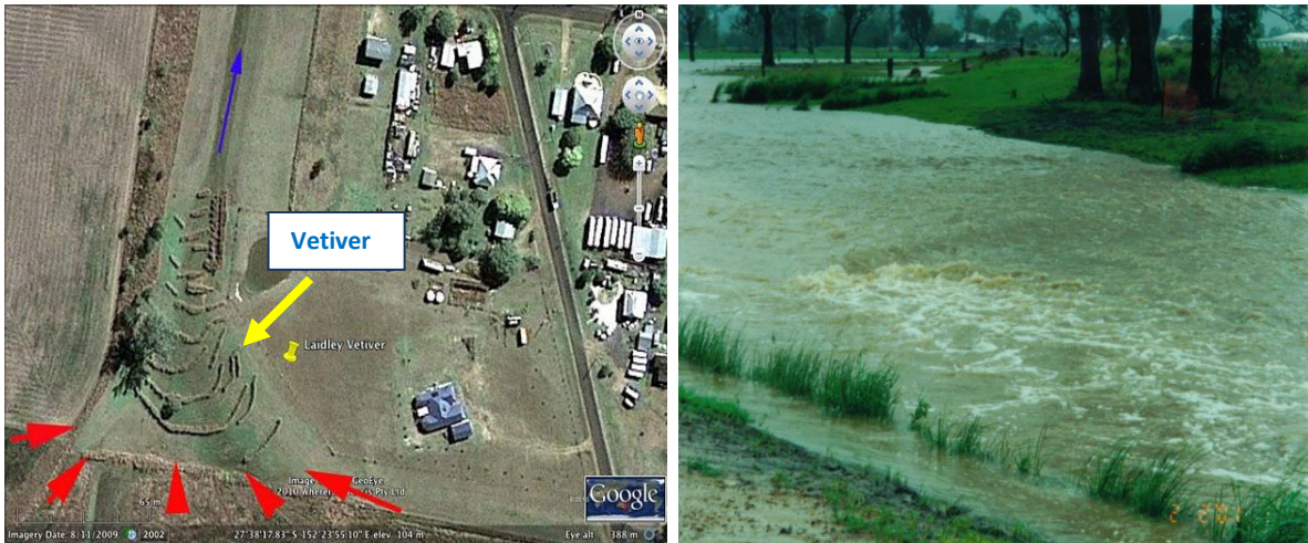
Layout of vetiver rows at the head of the drain and flood flow at 5m/sec
